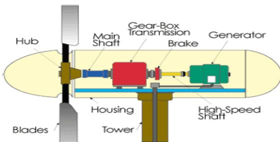
Figure1. The main components of wind turbine
