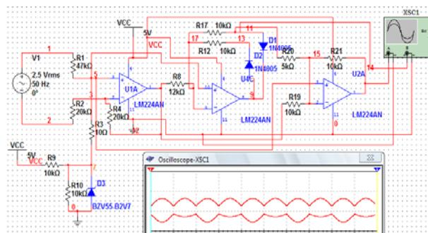
Figure 8. The proposed interface circuits for measuring dc voltage
