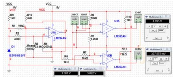
Figure 4. The proposed interface for measuring Temperature as digital value
