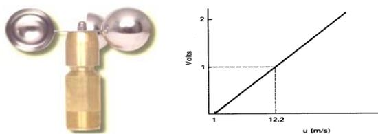
Figure 9. Classical anemometer
