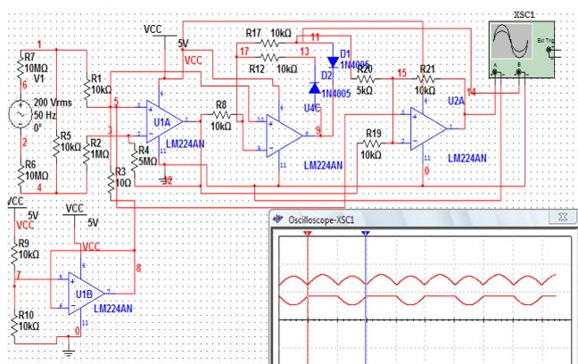
Figure 12. The proposed interface circuits for measuring Ac voltage without o/p filter
