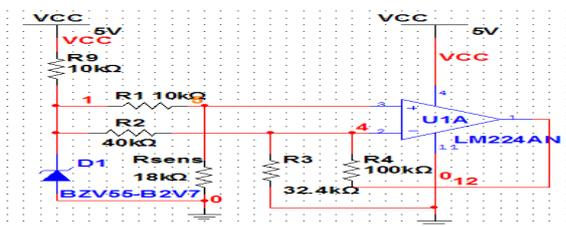
Figure 3. The proposed interface circuit for measuring Temperature as analogue value
