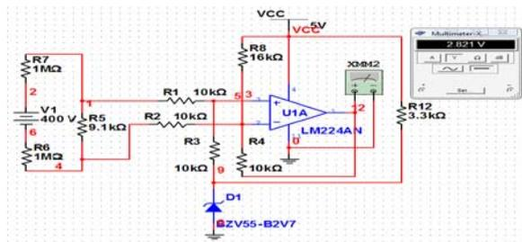
Figure 11. The proposed interface circuits for measuring high tension Dc voltage
