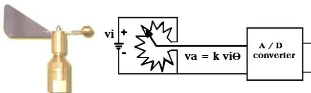
Figure 7. Wind direction sensors mechanical position to electrical output
