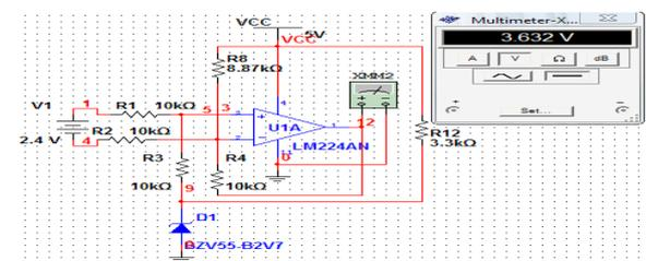
Figure 6. The proposed interface circuits for measuring dc voltage
