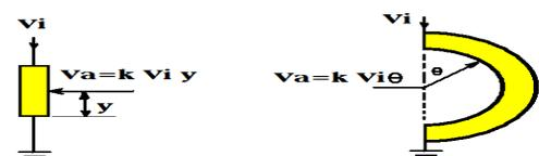
Figure 5. from left to right (a) Linear and (b) Rotary potentiometer
