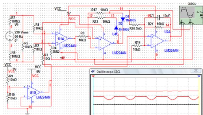
Figure 13. The proposed interface circuits for measuring Ac voltage with o/p filter
