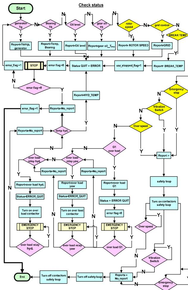
Figure 14. The proposed check status algorithm
