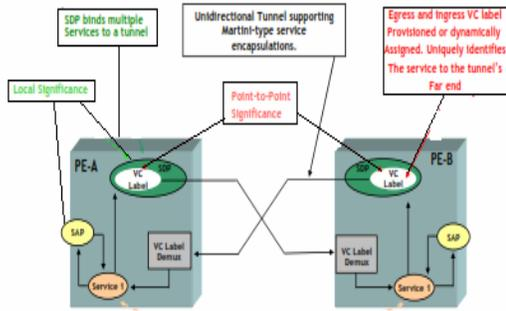
Fig 2 Layer 2 VPN working of MPLS (single node)
