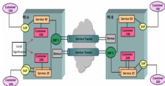
Fig. 3 Layer 2 VPN working of MPLS (multiple node)
