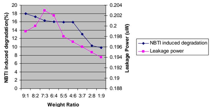
Fig.5. Leakage and NBTI-induced degradation after proposed algorithm under different weighted object function.
