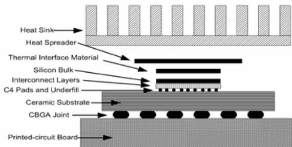
In three-dimensional IC's the heat dissipation pass through some of the interconnected layers having extremely low thermal conductivity materials. For this IC design micro fluid channel heat removal mechanism is proposed. In which the IC
