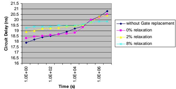
Fig.4. NBTI-induced delay after gate replacement under different delay relaxation at time 0.
