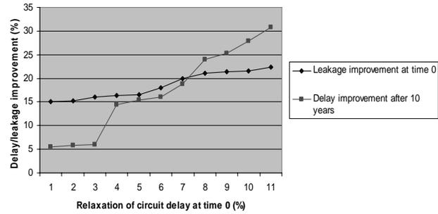
Fig.3. Leakage and NBTI improvement under different delay relaxation at time 0.
