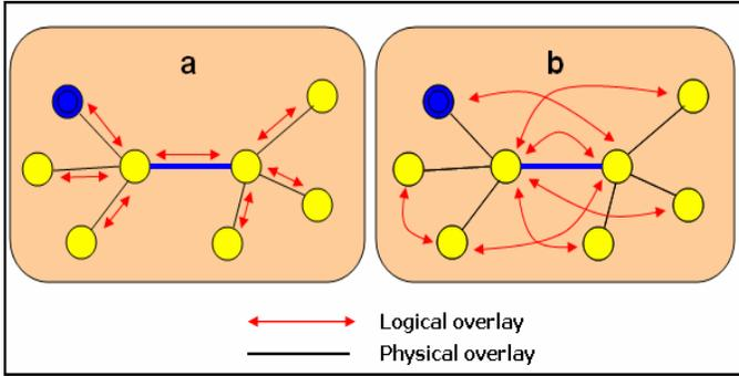
[Figure 2. Logical versus Physical Architecture]
