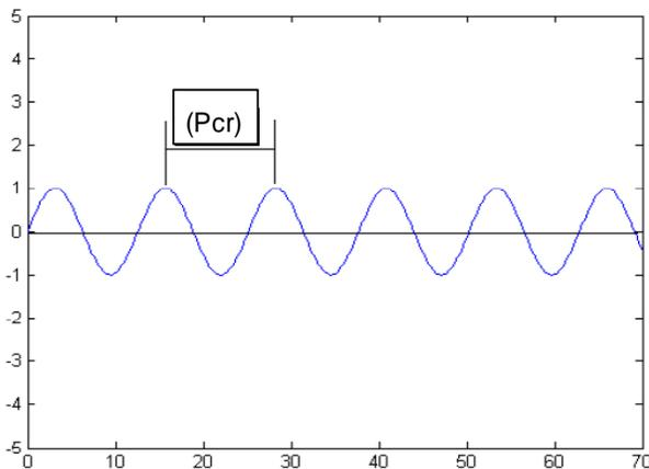
Figure 2. Illustration of Sustained Oscillation with Period  $P_{cr}$
