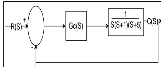
Figure 3. Block Diagram of Controller and Plant.
