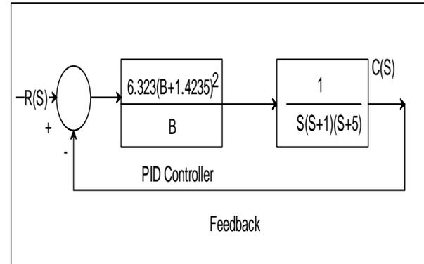
Figure 4. Illustrated the Close Loop Transfer function.
