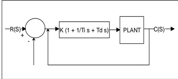
Figure 1. Block diagram of Continuous PID Controller.
