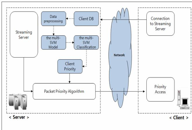
Figure 3. The Framework of the streaming server's user processing technique using Packet Priority Algorithm
