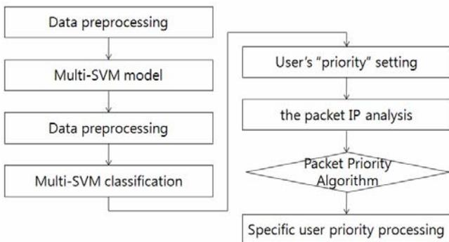
Figure 7. The work flow of the streaming server's data processing technique
