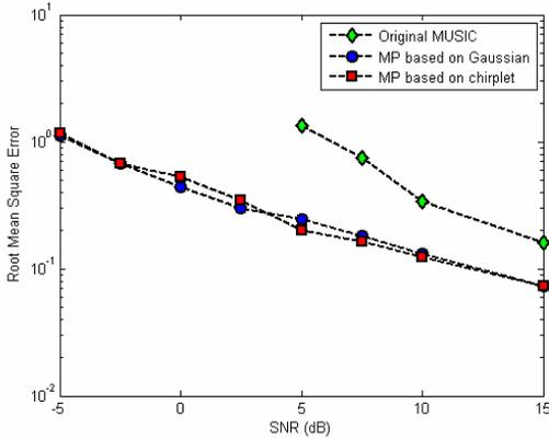
Figure 4. RMSE of DOA estimation for original MUSIC, and our proposed method. The impinging angle is  $10^\circ$  and  $20^\circ$  and the number of trial is 20, the number of snapshot is 101.
