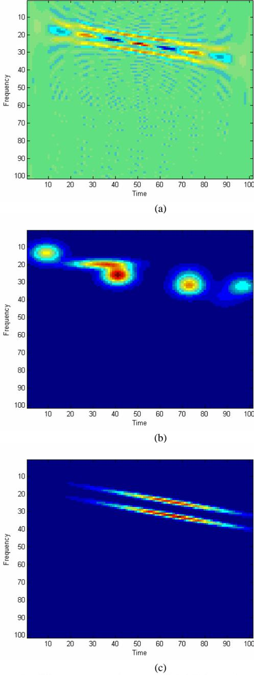
Figure 3. TF distribution of two parallel LFM signal, (a) WVD, (b) MP distribution based on Gaussian atom (decomposition number is 8), (c) MP distribution based on chirplet atom (decomposition number is 2).
