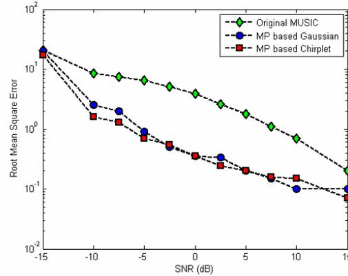
Figure 2. RMSE of DOA estimation for original MUSIC, and our proposed method. The impinging angle is  $10^\circ$  and the number of trial is 20, the number of snapshot is 301.
