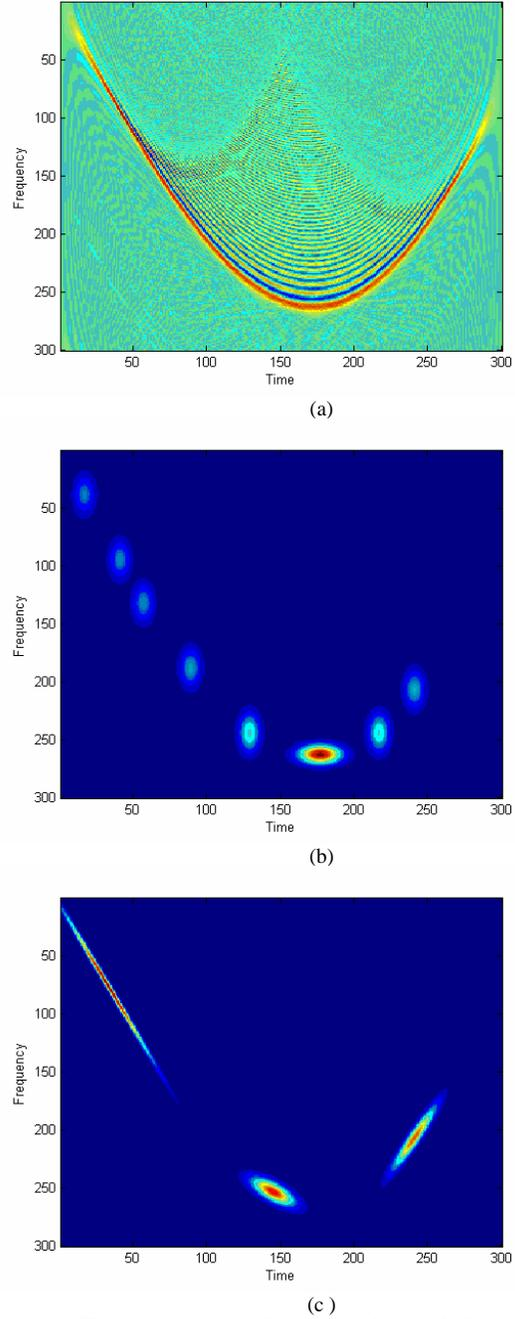
Figure 1. Time frequency distribution of polynomial phase signal, (a) WVD, (b) MP distribution based on Gaussian atom (decomposition number is 8), (c) MP distribution based on chirplet atom (decomposition number is 3).
