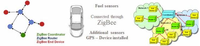
Figure 4. ZigBee network [14], a ZigBee Device Types, ZB Coordinator – 15.4 PAN Coordinator, ZB Router 15.4 FDD/Coordinator, ZB End device 15.4 RFD.
