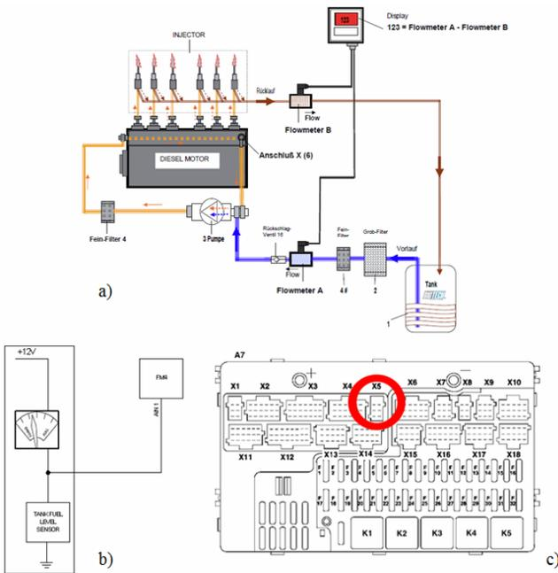
Figure 2. a) Bio-Tech flow meter [11], b) Taltonika fuel tank level sensor [2], c) X5 connector located in the fuse box for CAN wires.
