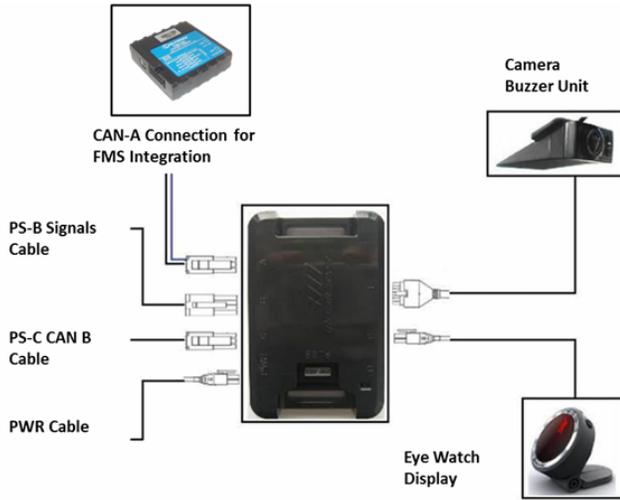
Figure 8. Collision Prevention System connection scheme.
