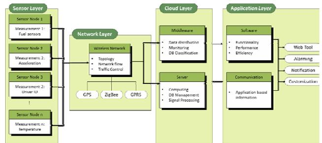
Figure 5. Diagram with information flow and how all layers that are related to one another and displayed on a single graphical interface to the customer.
