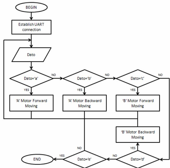
Figure 2. Flow diagram for microcontroller developed program
