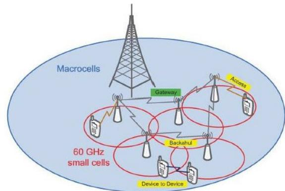
Fig. 1. Dense deployment of small cells in the 60 GHz band underlying the macrocell network [1]
